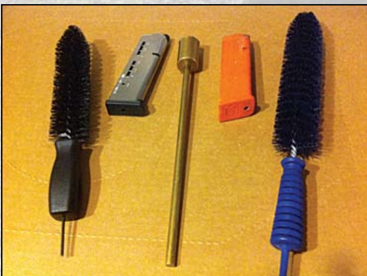
Magazine brushes and squib rods are important tools for the shooter and Safety Officer.
