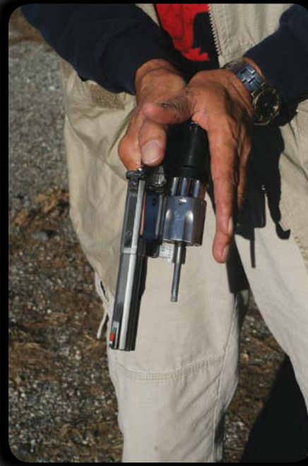
Dominant right hand maintains grasp on frame (thumb clear of cylinder) as supporting left hand slaps loader into cylinder.
